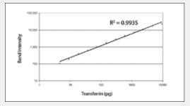
The dynamic range was determined using a serial dilution of Transferrin detected with a Cy5 labeled antibody. The dynamic range was linear over 3.3 orders of magnitude.
