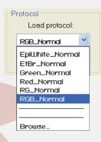
AlphaView Q simplifies the imaging process by allowing a protocol to be saved for a unique experiment. The protocol is recalled with one click and saves the user time by storing the light sources, filter settings and optimal exposure time.
