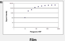
Comparison of FluorChem Q with film. A two-fold dilution of HRP conjugated antibody was spotted onto a membrane and imaged with the FluorChem Q and with film. Figure A) The response of the FluorChem Q to chemiluminescence signal was linear from 2.5 nanograms to 1.2 picograms, a dynamic range of 2083:1. Image exposure time was 6 minutes, and was captured using a 1X1 bin. B) Film exposure required 5 minutes to see a similar limit of detection, but showed rapid saturation of signal.
