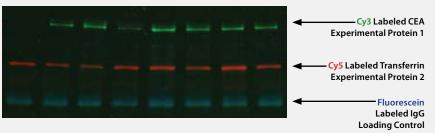
Composite image of a three-color fluorescent Western blot. Three different proteins, Transferrin, Carcino Embryonic Antigen (CEA), and IgG, were detected with fluorescently labeled antibodies, and imaged in three spectrally unique fluorescent channels. Imaging time was 24 seconds.
