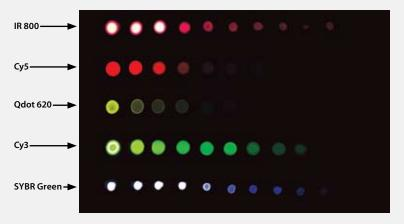
Five fluorescent dyes can be captured in one assay with the FluorChem Q. A different exposure time, excitation source, and emission filter was used for each dye.
