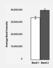
Uniformity of fluorescence imaging on the FluorChem Q. Two bands on one Western blot were imaged at 12 different positions within the FluorChem Q and quantified. The mean value and standard deviation for each band are shown. The CV for band 1 was 3.1%, and for band 2 was 2.7%.
