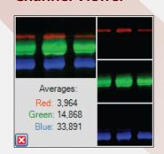
The unique channel viewer feature allows you to visualize all the features in your sample simultaneously as a three-color or single-channel image. If two bands overlap, you can see the contributions from each channel
